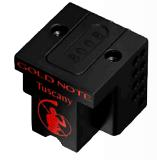
The Tuscany Red helped by its 200hm high internal impedance and the 0.4mV output level can be easily matched with any MC active phono preamp without Step-Up transformers.
